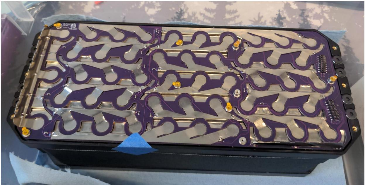
Figure 2.21: Nickel interconnect placed and soldered on carrier PCB
