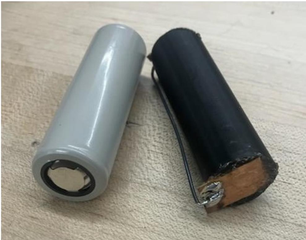
Figure 3.9: The constructed fake cell.
