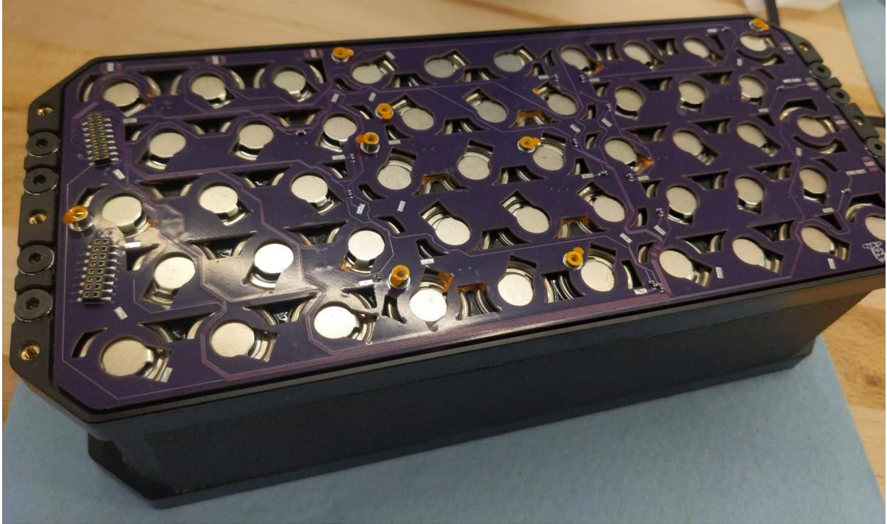
Figure 2.20: Carrier PCB installed on module.
