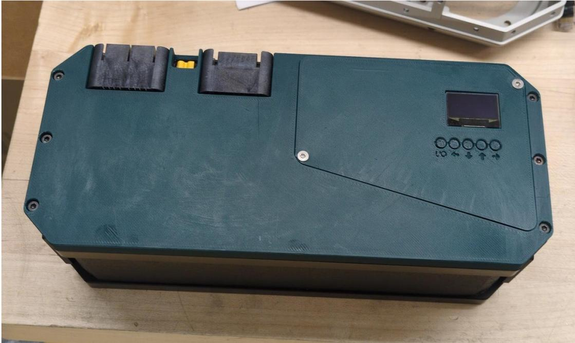
Figure 2.6: Final battery assembly
