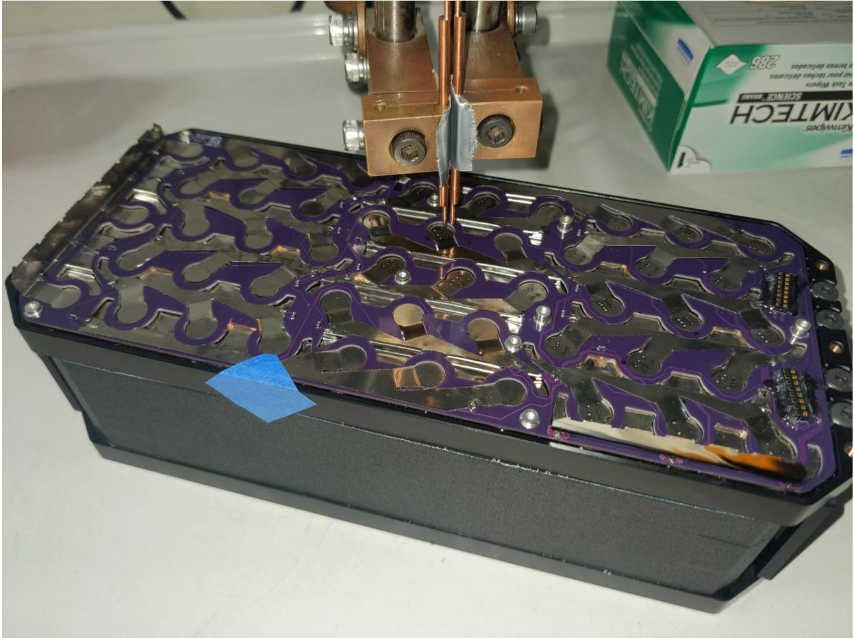
Figure 2.23: Each interconnect is spot welded by hand.
