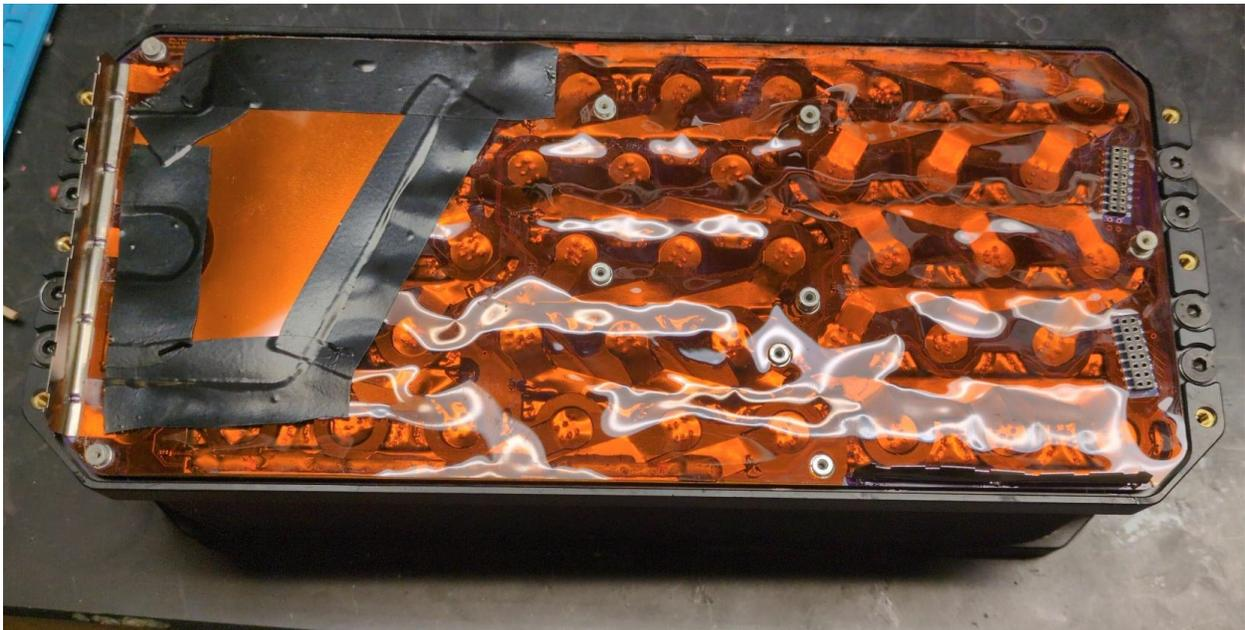
Figure 2.25: The final interconnect that folds over is soldered to the exposed interconnects and is insulated over.
