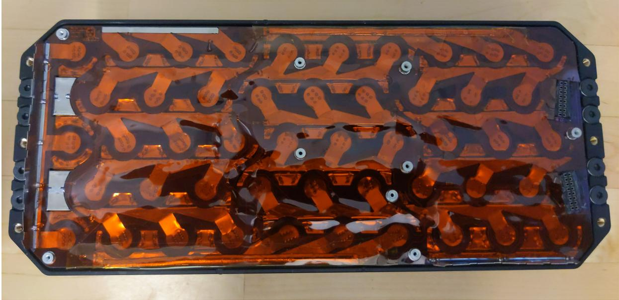
Figure 2.24: A layer of Kapton insulates the spot welded interconnects.
